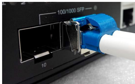
Figure 2.9 - LC Connector to the Transceiver
